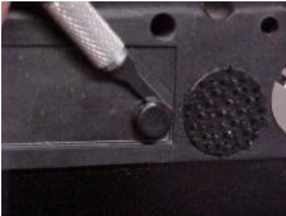
Using a good soldering iron and some solder wick, de-solder the old photocell and it can be pulled out of the front of the cluster (tip - put a little solder flux on the wick and it will work MUCH better).
