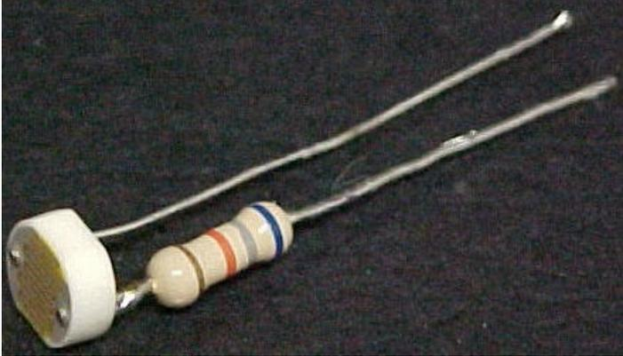
Then just insert the photocell/resistor assembly into the hole in the front of the cluster and push the leads through the holes in the LCD driver board. It's a little tricky to get the leads lined up with the holes in the PCB board. Again, it does not matter which lead goes to which hole in the PC board. Once the photocell/resistor combo is in it will look something like this:
