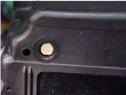
With the series resistor the cell will not sit all the way back in the hole in the front of the cluster. In this picture I used a 1/2 watt resistor (that's all I had). If you use a 1/4 watt resistor the photocell will be able to sit a little deeper in the hole.
