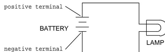
Since a simple DC lamp is nothing more than a resistor that emits light, we can show this same circuit using a resistor instead of a lamp:
