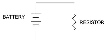
So lets give these components some values and analyze this circuit. We'll say the battery is 12V and the resistor is 10Ω.
