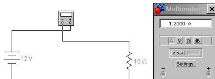
Obviously if a Voltmeter is placed across the resistor the reading will be 12V since it's basically connected directly to the battery's terminals. This can also be proved mathematically since  $V = RI$  we would multiply 10Ω by 1.2 Amps to come up with 12 Volts.
